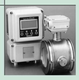
Both the converter and the detector provide the same features as the MagneW 3000 PLUS. High-performance EFTE lining models extend operating life in abrasive environments common in pulp and paper and mining applications to more than 15 times that of PFA linings.
