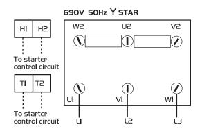
T1 and T2 = Thermistor connections H1 and H2 = A.C. Heater connections (Supplied on request)
