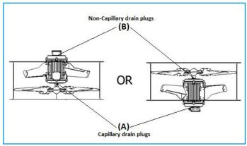
Figure 3. Vertical mounted axial fans.
