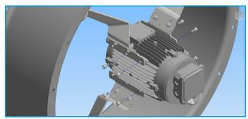
Figure 8. Removal all motor fixings.
