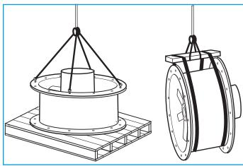
Figure 1. Correct method of lifting/removing from a pallet.
