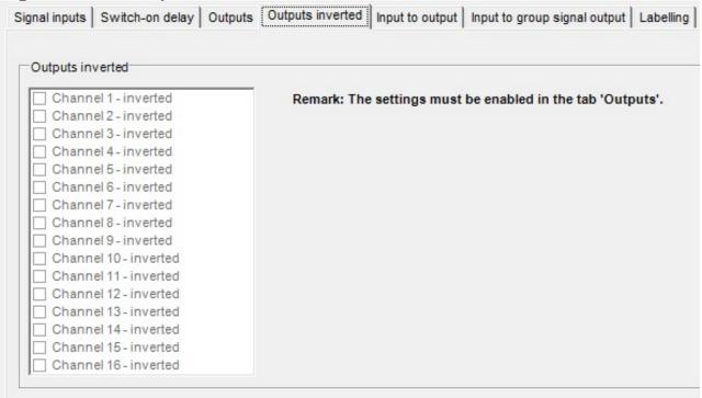
When activated "Outputs inverted" in the Register card "outputs", the outputs can be specified here to be inverted.
