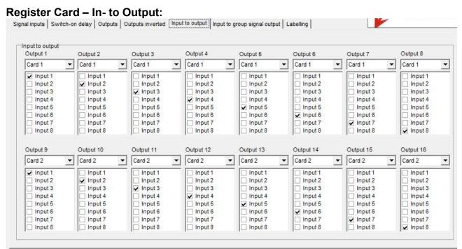
When activated "In- to Output" in the Register card "outputs", the input-output mappings can be made.
