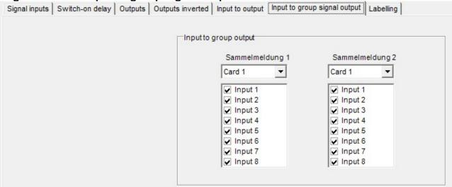
The selected inputs set the corresponding group alarm output.
