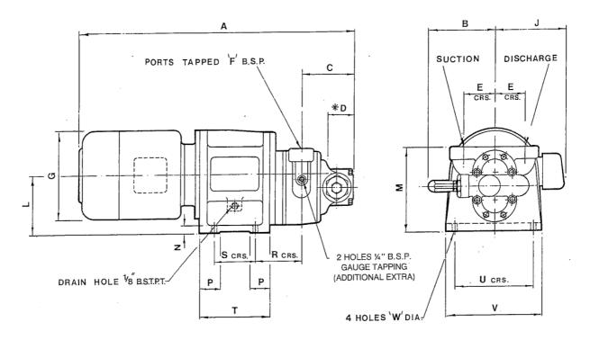
\* WHEN BY PASS IS NOT FITTED SUBTRACT DIMENSION  $\mathbf{\dot{D}}'$
