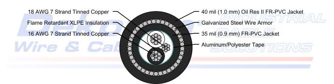
**Voltage Rating:** 300V UL PLTC/ITC **Temperature Range:** -20°C to 105°C
