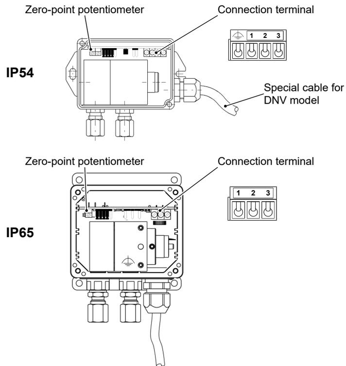
Fig. 7: Cable connection
