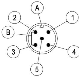
Fig. 8: M12 plug 5-pin+bridge
