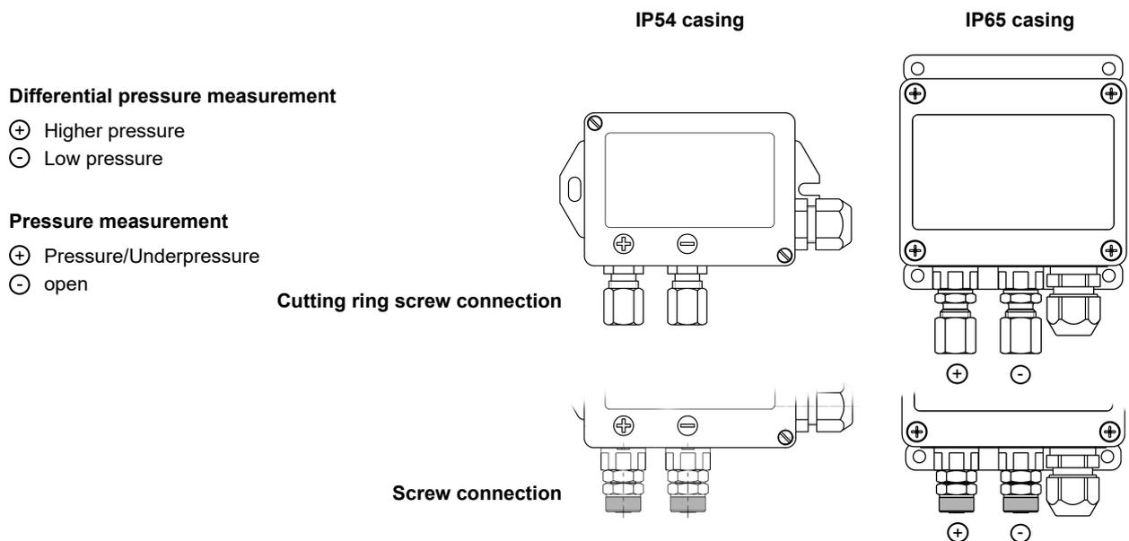
Fig. 5: Process connection
