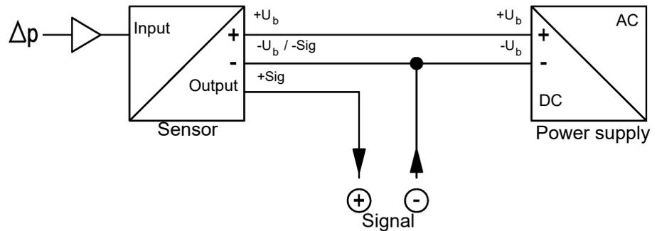
Fig. 6: 3-conductor circuit
