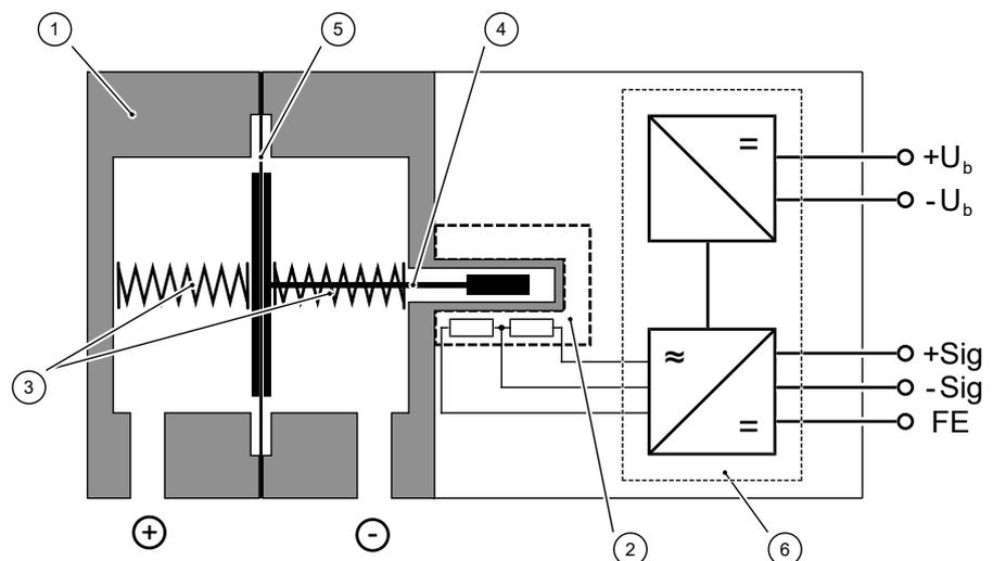
Fig. 4: Function diagram
