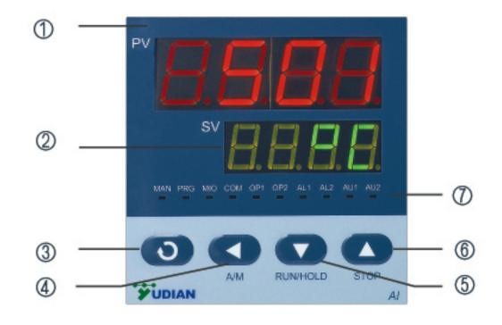
**Basal display status**: When power on, the upper display window of the instrument shows the process value (PV). This status is called basal display status. When the input signal is out of the measurable range (for example, the thermocouple or RTD circuit is break, or input specification sets wrong), the upper display window will alternately display "orAL" and the high limit or the low limit of PV.
